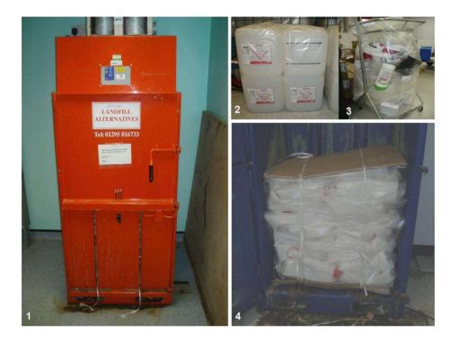
The machine (picture 1) is housed in the storage room adjacent to the main dialysis unit and measures approximately 6ft by 3ft by 3ft. An electronic machine was chosen ahead of pistondriven alternatives as it makes very little noise, an important consideration given the close proximity to a clinical area.
