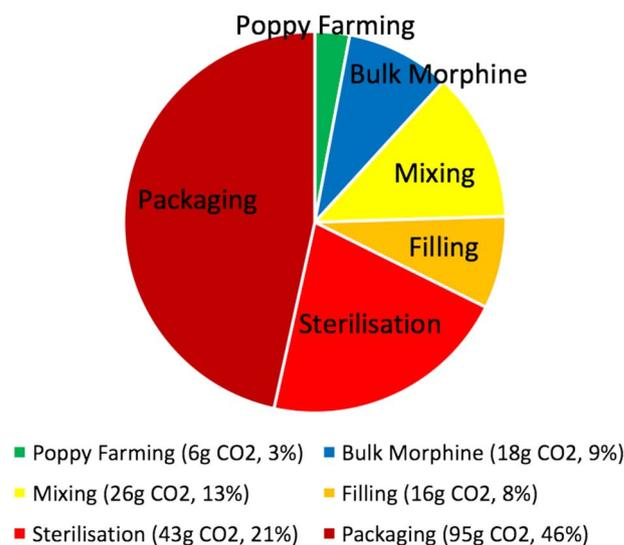
**Figure 2** Greenhouse gas impacts (g CO<sub>2</sub> and %) by stage of morphine's life cycle (205 g CO<sub>2</sub> total). The individual listing of the final steps in the process of morphine production (mixing, filling, sterilising and packaging) indicates that they are the most important contributors to morphine CO<sub>2</sub> emissions.
