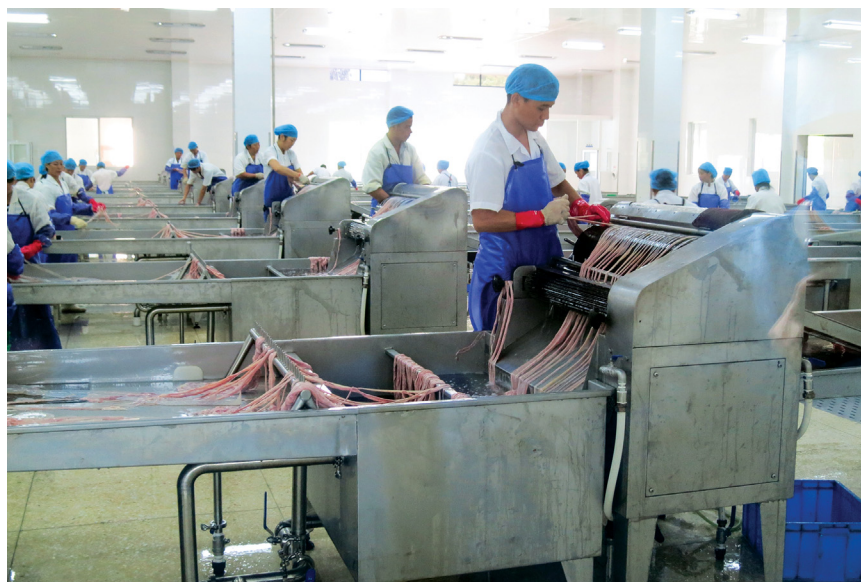
Figure 1. First step of producing heparin, separating mucosa from the pig intestines. Reprinted with permission from Chemical and Engineering News. Copyright ©2016 by the American Chemical Society. This image file first appeared in volume 94, issue 40 on October 10, 2016.
